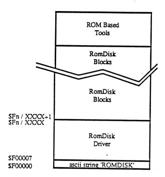
The initialization call made to the RomDisk driver should make a call to the ToolLocator to install the ROM based tool set extensions. This then allows the tool locator to dispatch to the ROM based tool set extensions directly rather than down loading the tool set to RAM.
