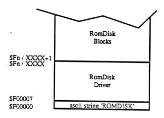
It is possible to use the expansion ROM for both a RomDisk and ROM based extensions to the tool set by partitioning the ROM into three areas (Driver, Blocks and Tools) as shown below:
